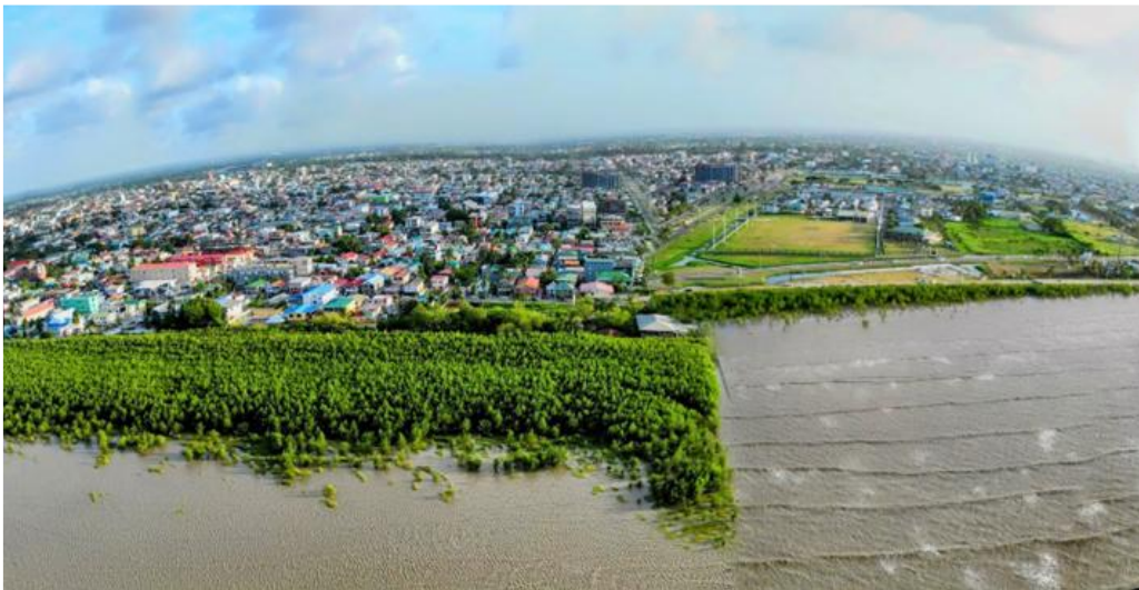
Georgetown, Guyana's mangroves provide crucial coastal resilience. This photo clearly shows settlement established along the mangrove coast where waves are weaker. In stark contrast, the area without mangroves lacks settlement, exhibits significant erosion, and is battered by stronger waves, increasing flood risk. (Photo: Anupam Anand/GEF IEO)
