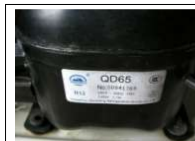
Figure 70: CFC-12 compressor from China. Savodo Teknika, Uzbekistan
