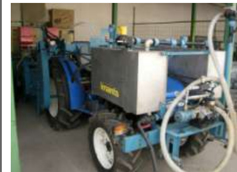
Figure 21: Rotary spader adapted for use in glasshouses with nematocide as liquid (front tanks) or granules (red rear tanks). Zephyr, Hungary.
