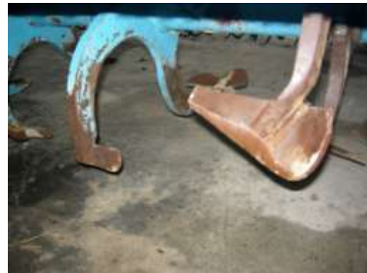
Figure 38: Spader showing nematocide bins (red), and details of spades that are damaged by rocks in soil. Solfum, Poland.
