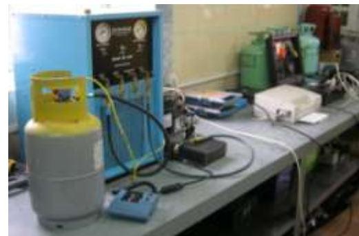
Figure 49: Equipment for recovering ozone-depleting substances. Podolskorgtechnika, Moscow.
