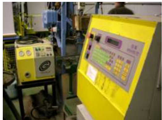
Figure 58: Gas charging equipment. Iceberg, Smolensk.
