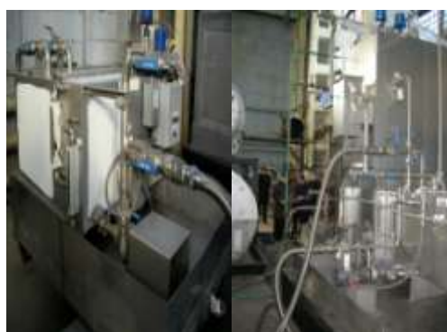
Figure 30: Unused methylene chloride equipment purchased to replace CFC-113 solvent. Pavlodar Chemical Company, Kazakhstan.
