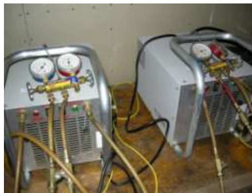
Figure 68: ODS reclamation equipment and storage cylinders (above), and recovery equipment (below). Shark Shaboda, Uzbekistan.
