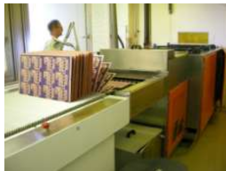
Figure 18: Stripmaster equipment with non-ODS solvent. Hitelap, Hungary.
