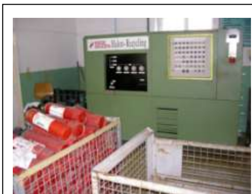
Figure 12: Halon cylinders ready for halon decommissioning (red), with Kidde-Deugra halon recovery and reclamation equipment (green). Fajro, Hungary.
