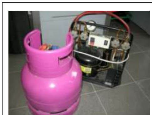
Figure 2: Equipment for recovery of ozone-depleting substances. Institute for Refrigeration and Air Conditioning, Sofia, Bulgaria.
