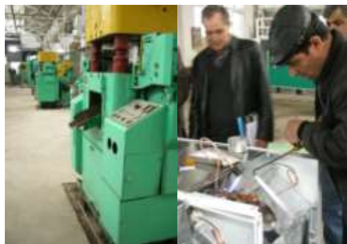
Figure 71: Template unit for cutting out door lining (left), welding compressor circuit to compressor (right), and finished refrigerators (below). SINO, Uzbekistan.
