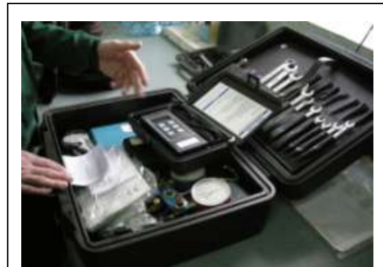
Figure 48: Set of servicing tools supplied for technical work on refrigeration and air conditioning equipment in the Russian Federation. Podolskorgtechnika, Moscow.
