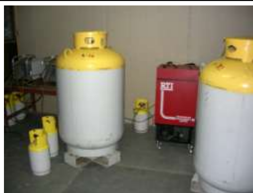
Figure 68: ODS reclamation equipment and storage cylinders (above), and recovery equipment (below). Shark Shaboda, Uzbekistan.
