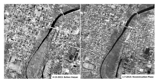
Figure 5. Remote Sensing analysis of the municipality of Tanauan (Leyte, Philippines) before and after Typhoon Haiyan to assess disaster damage and recovery using Geoeye and WordView VHR satellite imagery. In January 2014 large parts of the municipality are uninhabitable. Machine learning algorithms can be used to train for the detection of structural features such as temporary shelters (lower left corner). (Source: Authors' own draft)
