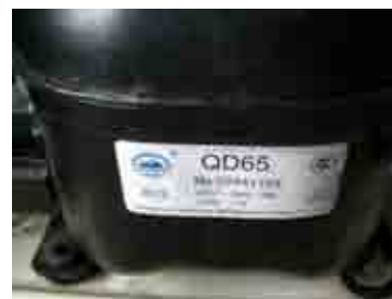
Figure 51: CFC-12 compressor from China. Savodo Teknika, Uzbekistan
