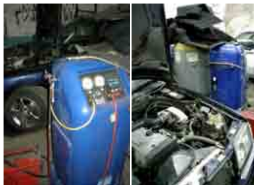
Figure 27: ODS recovery equipment from mobile air conditioning. Auto Klimat, Kazakhstan.
