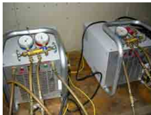
Figure 50: ODS reclamation equipment and storage cylinders (above), and recovery equipment (below). Shark Shaboda, Uzbekistan.
