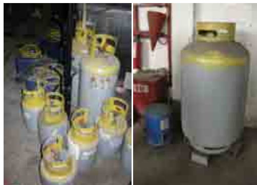
Figure 26: Smaller cylinders and equipment (blue) used for ODS recovery and storage (left) with unused large tank (right). Polair, Kazakhstan.
