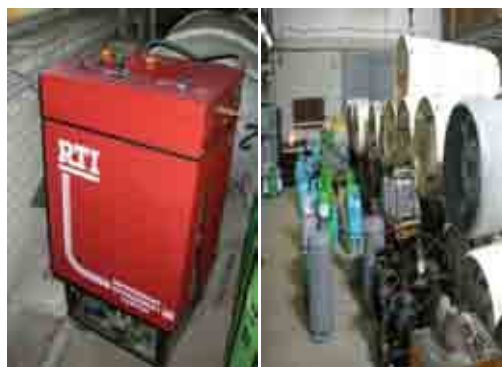
Figure 30: RTI recovery and recycle equipment (left) and stored ODS (right). Revers Refrigeration, Latvia.
