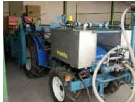
Figure 23: Rotary spader adapted for use in glasshouses with nematocides as liquid (front tanks) or granules (red rear tanks). Zephyr, Hungary.
