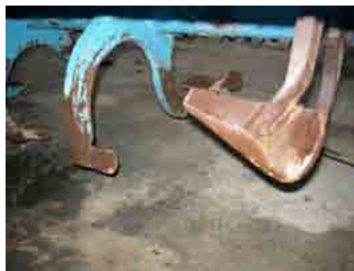
Figure 36: Spader showing nematocide bins (red), and details of spades that are damaged by rocks in soil. Solfum, Poland.
