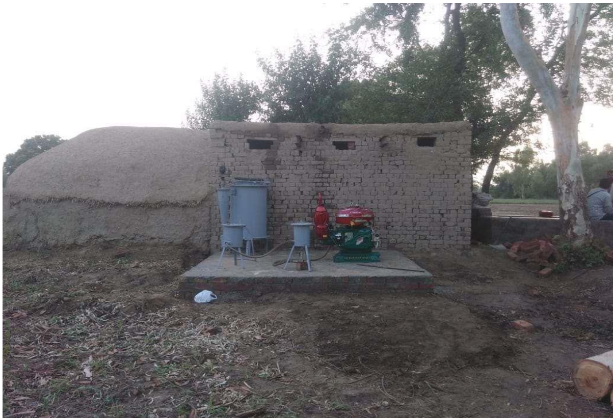
Figure 10: The project funded Tawanai Solutions 25kW gasifier and diesel motor for rural water pumping
