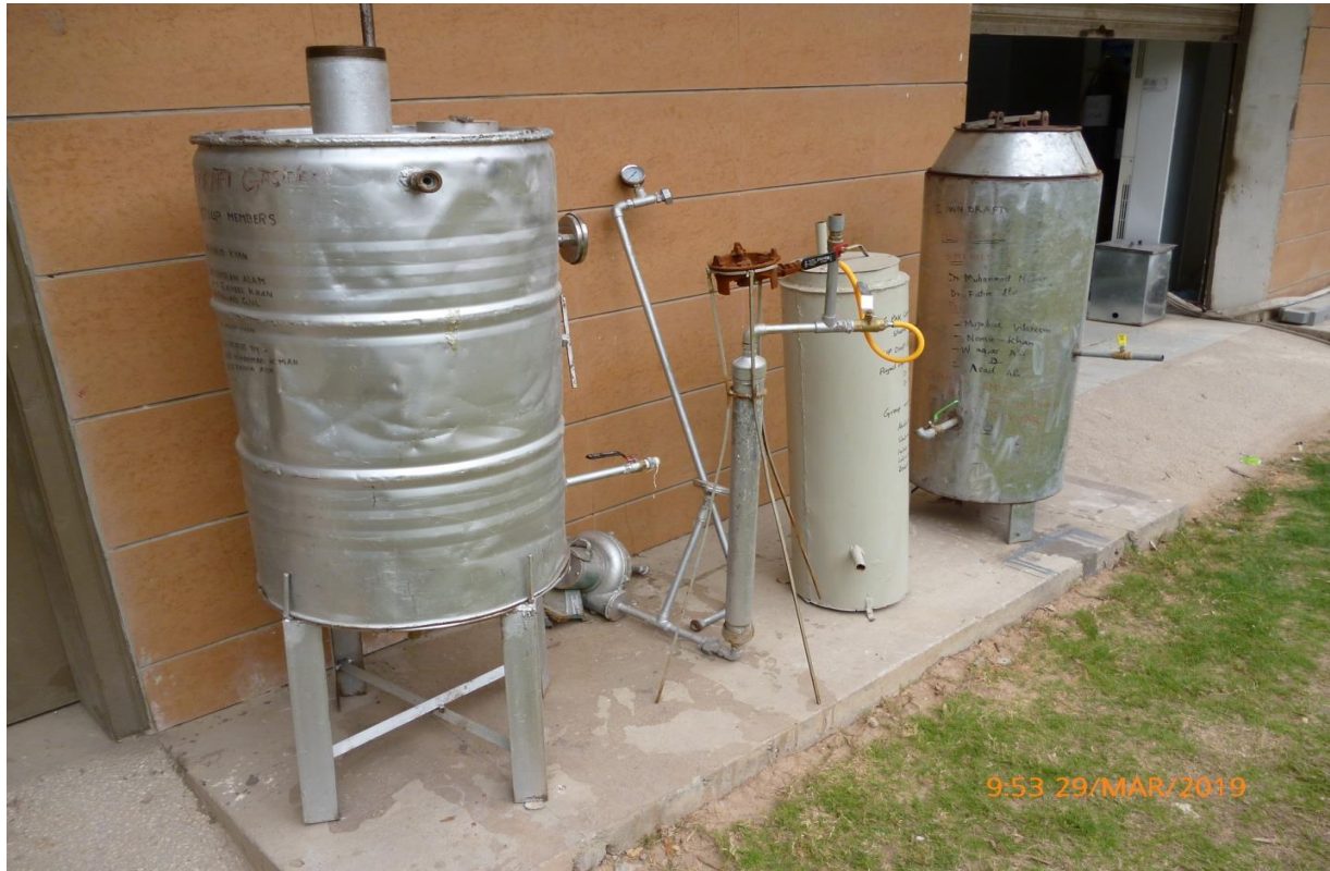
Figure 9: Faisalabad Agricultural University Student Designed Demonstration Gasifier
