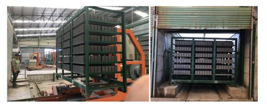
Concrete Brick production and curing using solar energy and heat-trapping system
