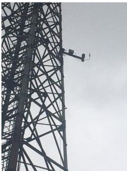
An AWS fixed to an Africell cell-phone tower in Bo
