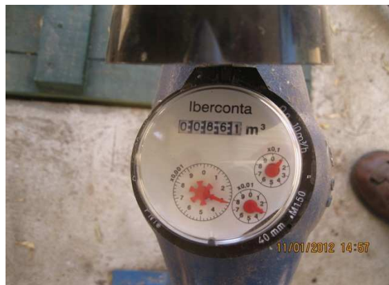
Water pumped meter (accumulative of 861 m 3 , 0.79 m 3 /per day average for 3 years)
