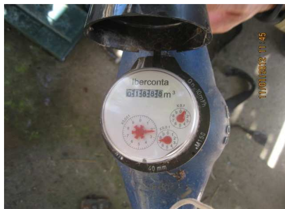
Water pumped meter (accumulative of 1888 m³, average 1.7 m³/per day for 3 years)
