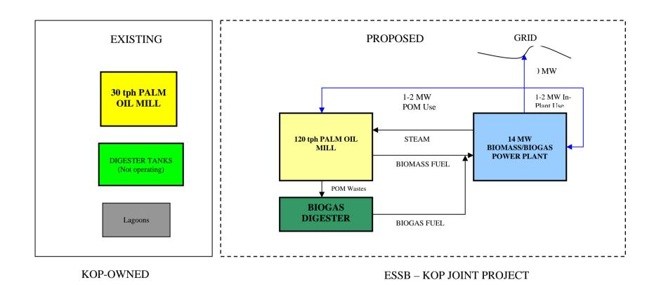
Figure 1. Existing POM owned by KOP and the Proposed New POM and Biomass Power Plant Complex
